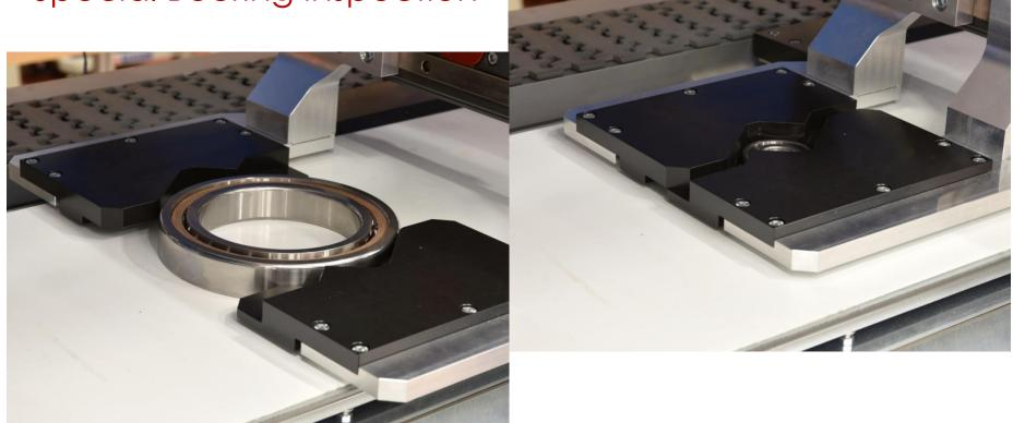
Automatical adjusting for different diameter: both **mechanically**...
